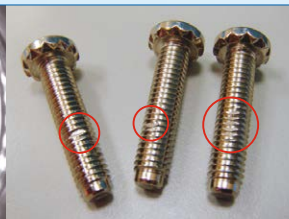
360° Degree Thread Damage Inspection (Customized)
