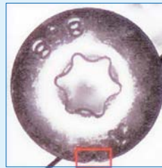
Kopfriss Head Crack
